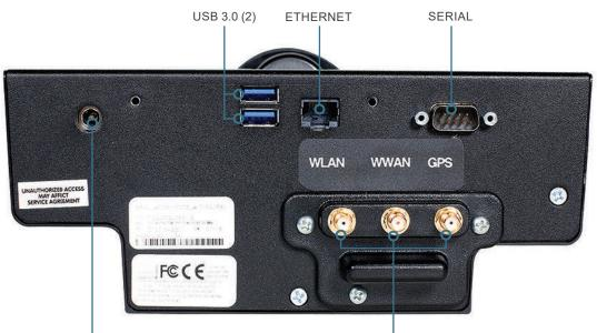
POWER SUPPLY INPUT RF (SMA) Antenna Pass-Through for GPS, WLAN and WWAN
